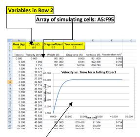
Velocity vs. Time Graph: Students alter the variables in row 2 and observe the immediate response in the graph. They learn by experimenting on each variable scientifically and quantitatively model everyday objects of all shapes and sizes falling through air.
